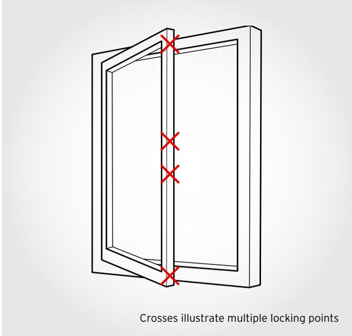
Strictly speaking a multi-point locking system can be any locking system that has more than one latch or locking point. The better systems are likely to have shoot-bolts at the top and bottom and a combination of hooks, latches, mushroom cams and/or roller cams along the opening side of the window or door. These locking points should ideally move in opposing directions.
